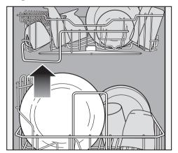
The stay at the front of the upper basket determines the max. height permissible for items placed in the lower basket to ensure they do not impede the movement of the middle spray arm.
